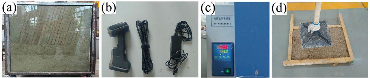
Figure 2. Test instruments and equipment: (a) The self-made movable model box; (b) 3D laser scanner and its supporting equipment; (c) Constant temperature blast drying oven; (d) Earth rammer.
