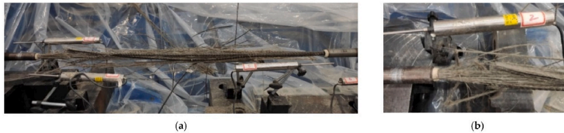
Fig. 18. Fracture of the BFRP tendon: (a) failure mode; (b) anchor without any slip [181].
