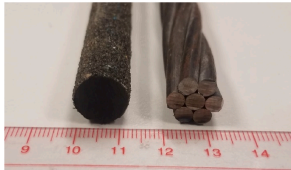
Fig. 20. CFRP and Steel tendon [198].
