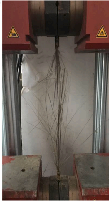
Fig. 19. The ultimate failure mode under fatigue test [57].
