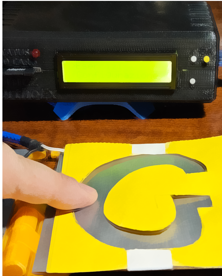
Figure 7. E2 exercise type in which the subject follows the shape of a letter (in the shown example the letter G) without losing contact with the capacitive sensor (metal part).
