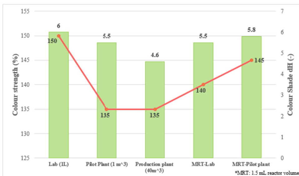
Fig. 4 Pigment quality: scaling-up (batch synthesis) vs. numbering-up of CPC-microreactors for small-scale production of a yellow azo pigment. Adapted from source [26]
