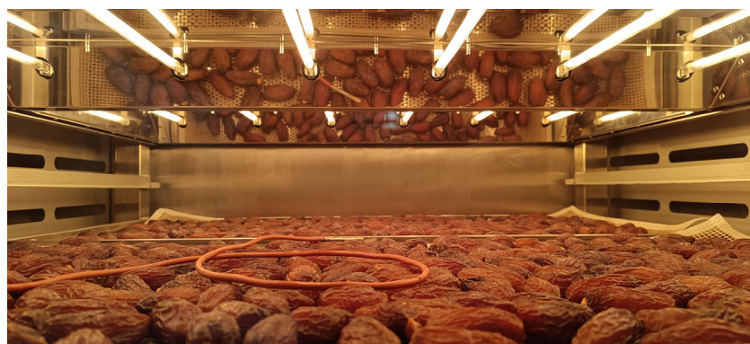
Figure 2. Illustration of infrared drying of ‘Mejhoul’.
