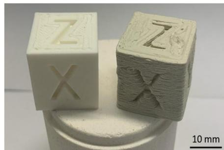
**Figure 6.** Print quality of calibration cubes in PLA (left) and 50%  $\text{Al}_2\text{O}_3$ /50% PLA (right) [24].
