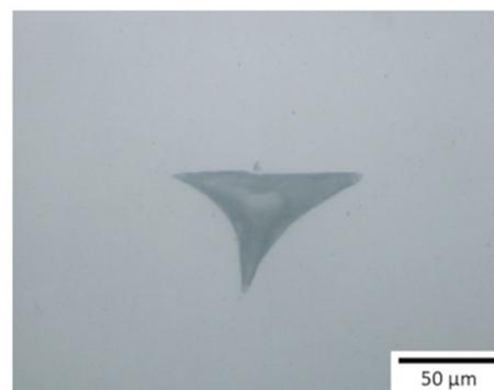
**Figure 11.** The printing process generated residual pores after MW 25 °C/min (adapted from [30]).
