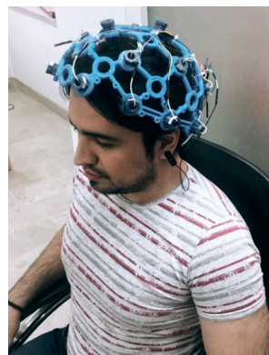
Figure 3. Recording of EEG signals using Open BCI modules on one of the participants.
