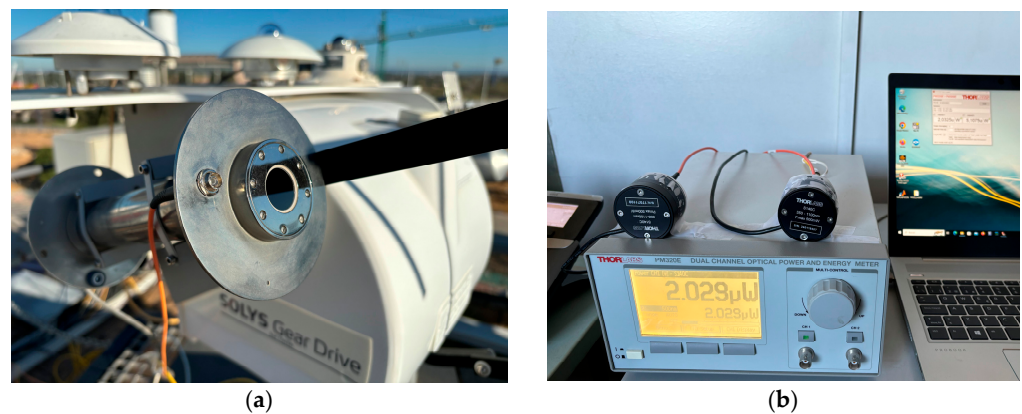
Figure 5. Experimental assembly for the proof of concept of the proposed instrument: (a) optical fiber and commercial pyr heliometer installed in a sun tracker; and (b) silicon photodiodes and an optical power meter, plus a computer for data acquisition.
