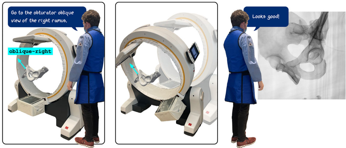
Fig. 1. Our system allows a user to control independent axes of a robotic X-ray system, the Brainlab Loop-X, using spoken natural language. Patient-specific views, such as the obturator oblique, are supported via automated image analysis
