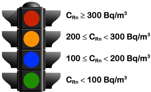
Figure 2. Traffic light for assessment of radon concentration results (Hernández Gutiérrez et al., 2019).
