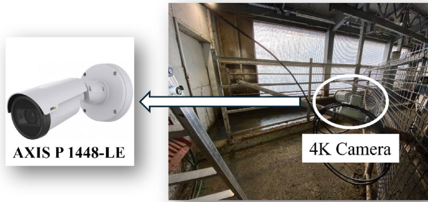
Figure 4. Camera configuration for monitoring lane A in the cattle Farm and camera type of 4K camera usage in cattle farm.
