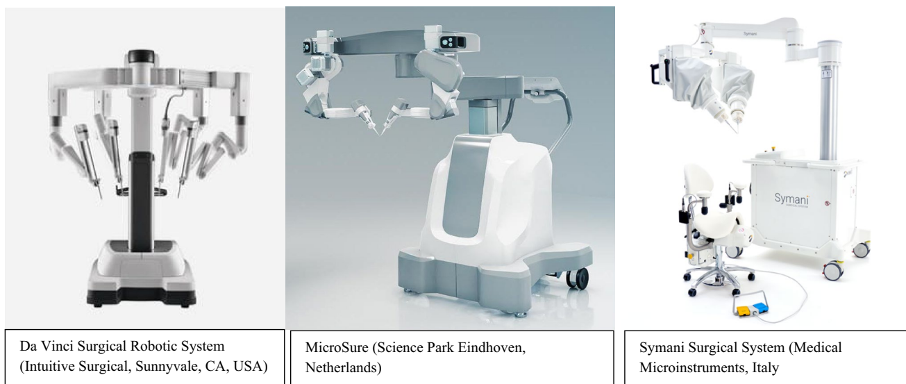
Fig. 1 Robotic equipment utilised within clinical practice. All three are controlled by a separate master console
