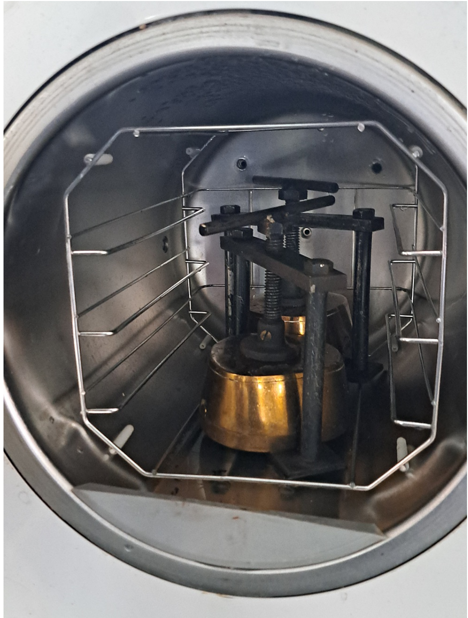
FIGURE 2: Denture flasks kept inside the pre-heated autoclave for autoclave curing
