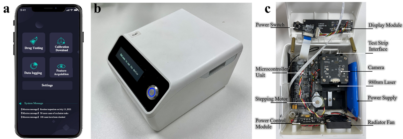
Fig. 5. Actual development of a transfer learning-based quantitative detection system for UCNP-LFAs. (a) Mobile phone application matched with the device, which can control the self-test and operation of the device through communication with the device, and can display the detection results in real-time, (b) UCNP-LFAs quantitative detection device based on transfer learning, which is portable and highly accurate due to the introduction of transfer learning, and does not need to rely on computing units with high computing power, with data localization being able to solve data privacy problems, and (c) the actual internal structure of the assay instrument.
