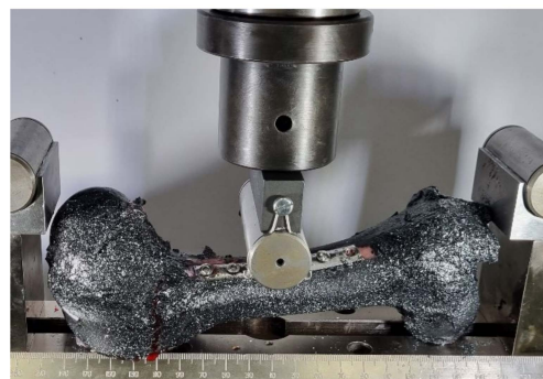
Figure 9. Application of concentrated vertical transversal load on reinforced bones.
