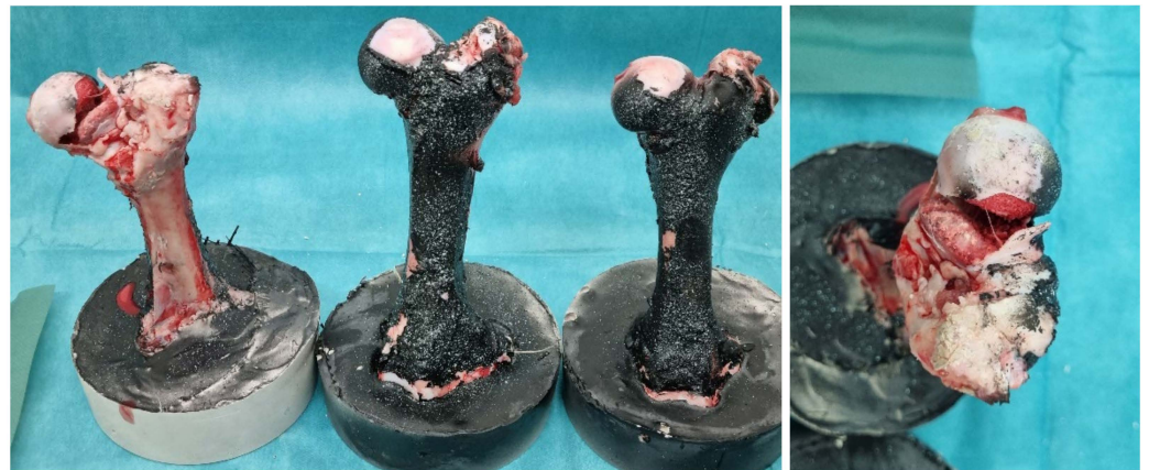
Figure 11. Femur bones without strengthening after the pressure test.
