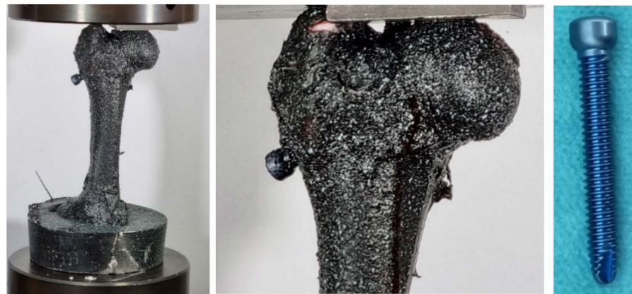
Figure 5. Strengthening titanium screws inserted in femur head.
