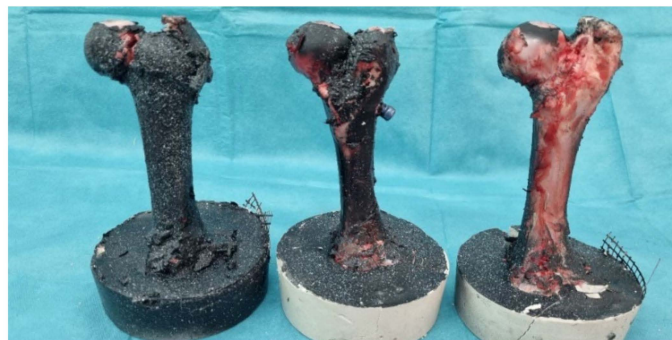
Figure 13. Femur bones with strengthening after pressure test.
