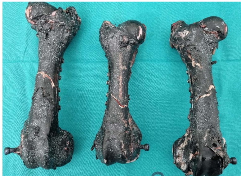
Figure 17. Femur bones with strengthening after three-point bending test.
