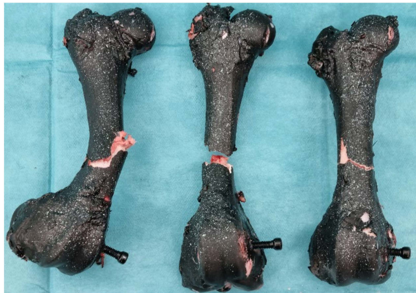
Figure 15. Femur bones without strengthening after the three-point bending test.
