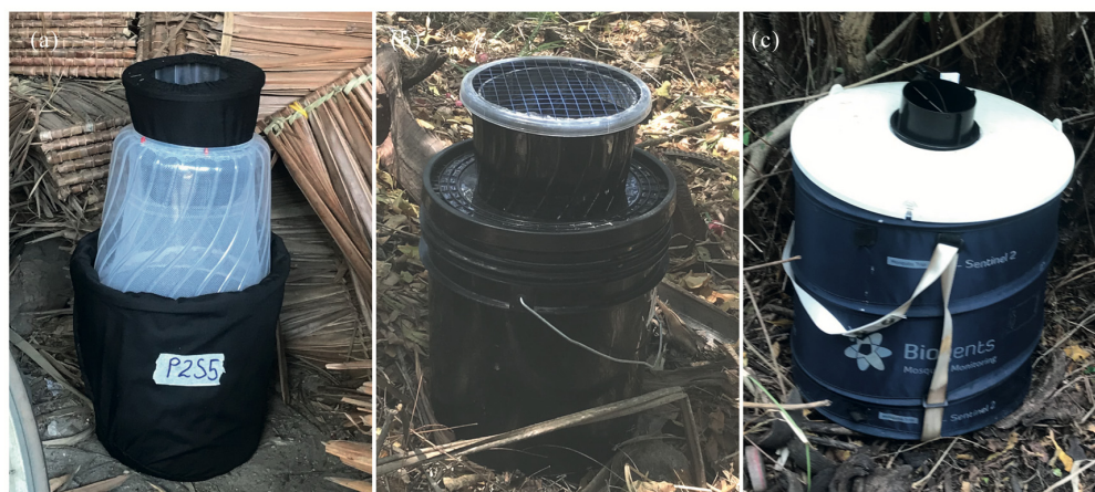
Figure 1. Mosquito traps. (a) Gravid Aedes trap (GAT), (b) Autocidal Gravid Ovitrap (AGO), and (c) Biogents Sentinel Trap (BGS).
