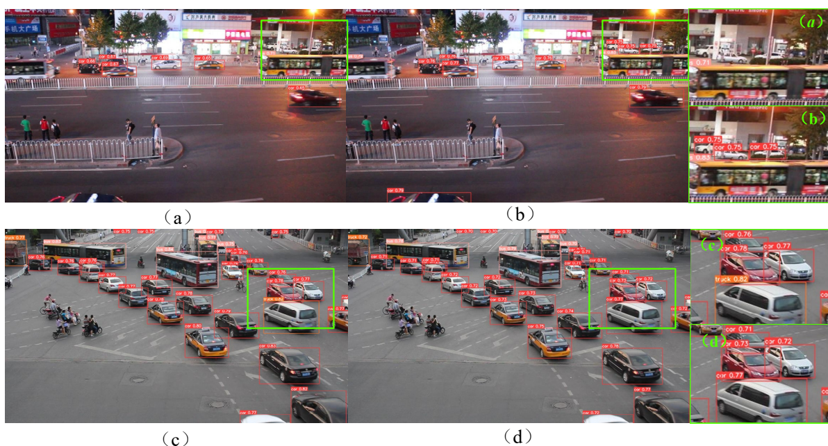
Figure 7. Comparison of detection results between YOLOv5s and IBi_YOLOv5s algorithms in dim lighting environments at night and street environments with a large number of vehicles: YOLOv5s (left); IBi_YOLOv5s (right). (a–d) represent vehicle detection scenarios in different situations.
