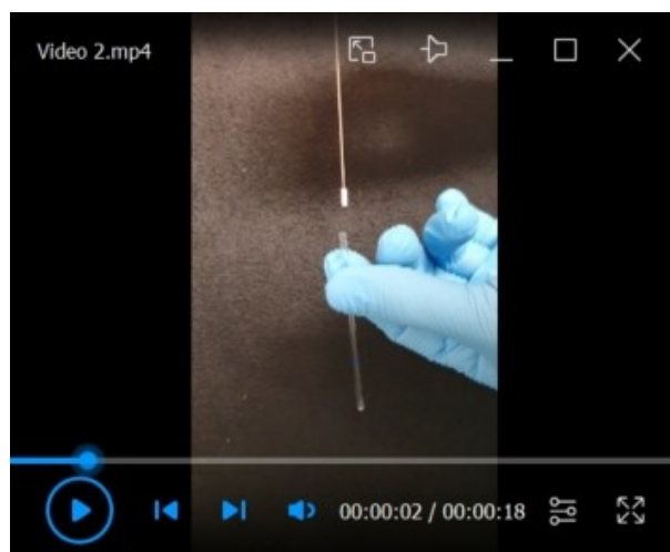
Video 2. Assembly of the modified Petri dish. This video shows how to assemble the plunger and capillary and how to connect them to the modified Petri dish. The plunger is inserted into the capillary,
