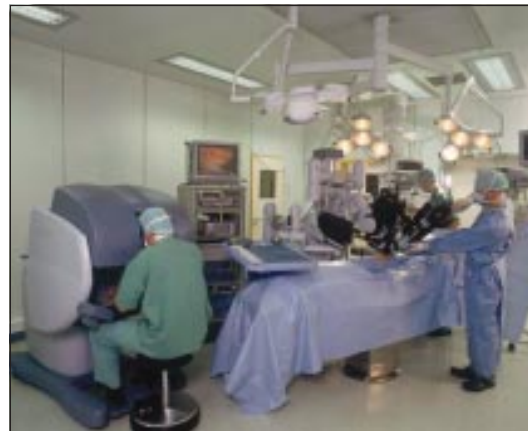
Fig 3 The da Vinci Surgical System (Intuitive Surgical, California, USA) for performing minimally invasive surgery. The surgeon sits at a control console with 3D visualisation of the surgical field and the robotic surgical instruments (reproduced with permission)
