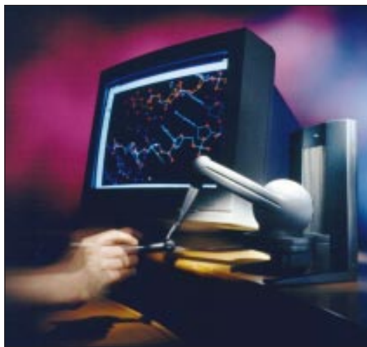
Fig 2 The PHANTOM haptic feedback device (SensAble Technologies, Cambridge MA, USA). The user holds a small stylus and explores, in this case, a 3D virtual molecular structure. Each time the 3D cursor makes contact with part of the structure, small motors work in tandem to restrict the movement of the stylus, thereby creating a sense of touch (reproduced with permission).
