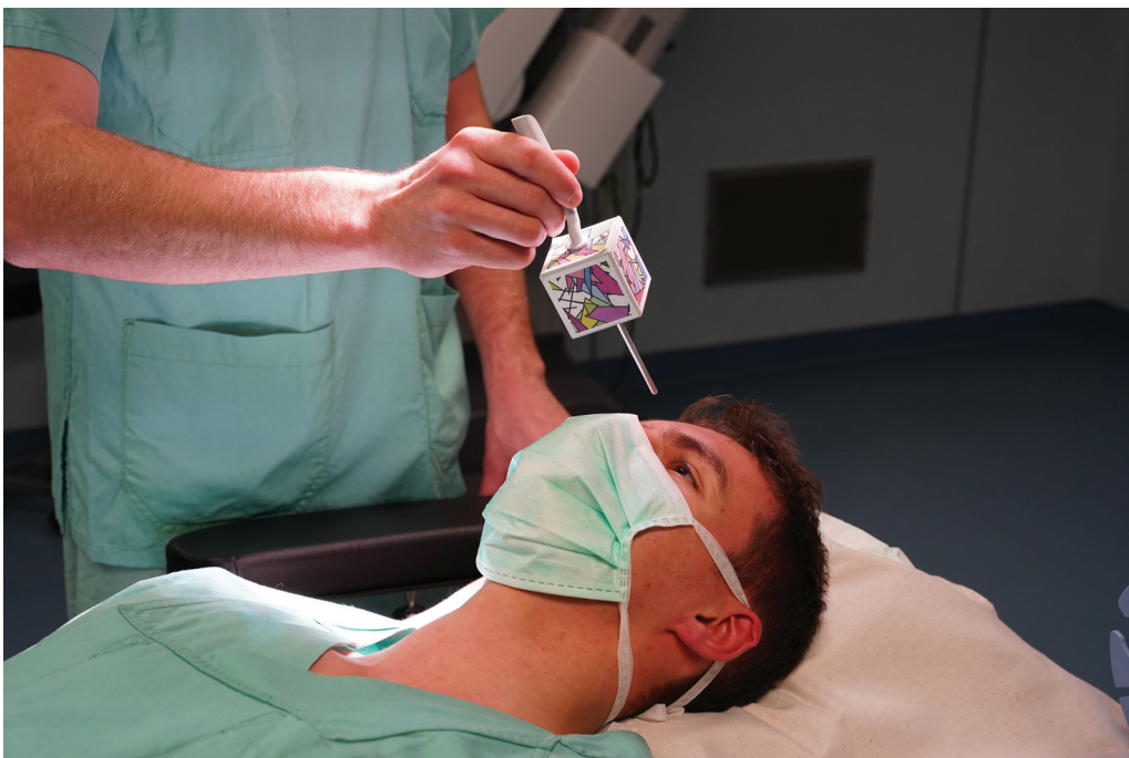
Fig. 2 The surgeon moves the surgical pointer to the points of interest at the patient. The colored pattern on the cuboid tracker is detected by the sensors of the HoloLens 2.
