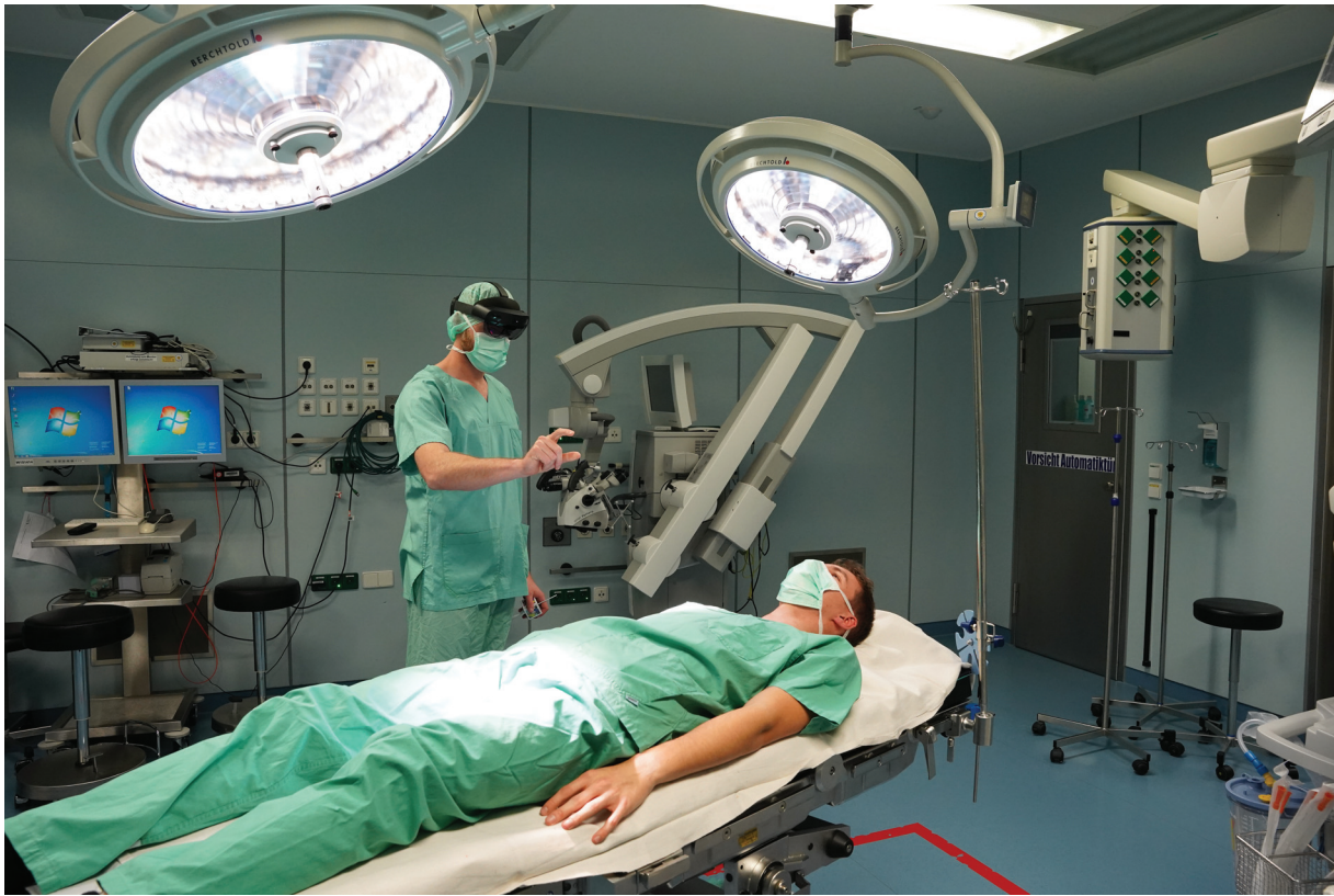
Fig. 1 Realistic test scenario inside an operating room. The surgeon interacts with his fingers through the menu of the navigation software.
