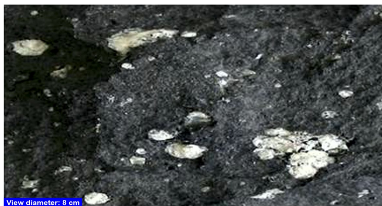
Figure 1. A sample of andesite (dark groundmass) with zeolite-filled amygdaloidal vesicles.
