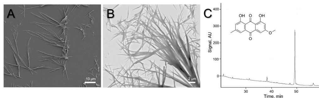
Figure 4. Visualization of parietin crystals using SEM (A) and TEM (B). HPLC elution profile of acetone extract from X. parietina with a major peak corresponding to parietin (C). Inclusion: the chemical structure of parietin (1,8-dihydroxy-3-methoxy-6-methyl-9,10-anthraquinone).
