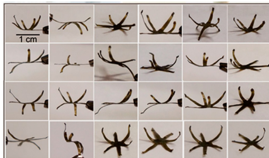
Figure 9. Liquid crystal–vitrimer/carbon nanotube composites reshaped into various 3D structures. Adapted from Ref. [77] with permission, Copyright 2016, American Chemical Society.
