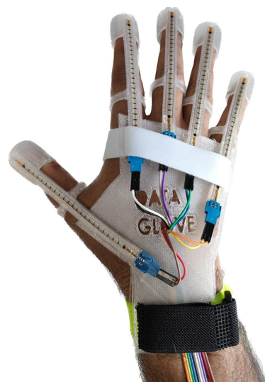
Figure 1. The 3D-printed data glove setup fabricated with the sensors.
