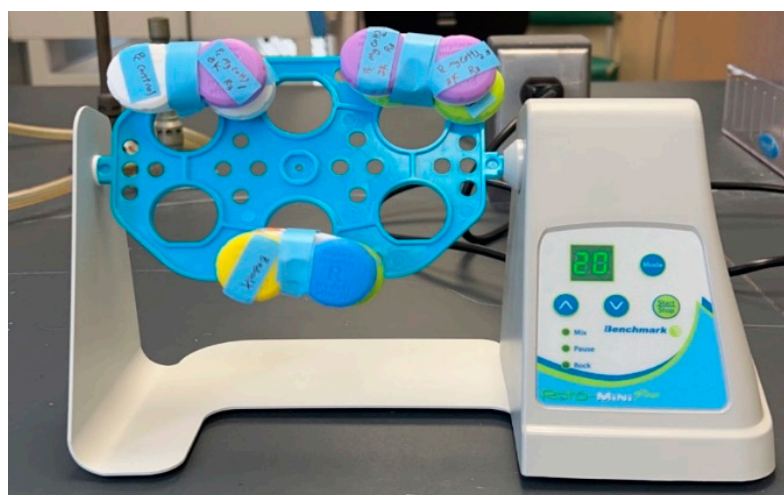
Figure 5. The pods were attached with tape to the mini rotator device for consistent agitation of the bacterial broth and surface renewal of the disks inside the pods. The blue tray holding the pods rotates around the horizontal axis. Reprinted from Ref. [26].
