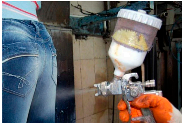
Figure 1. Classical human-based chemical spraying process on denim textile.
