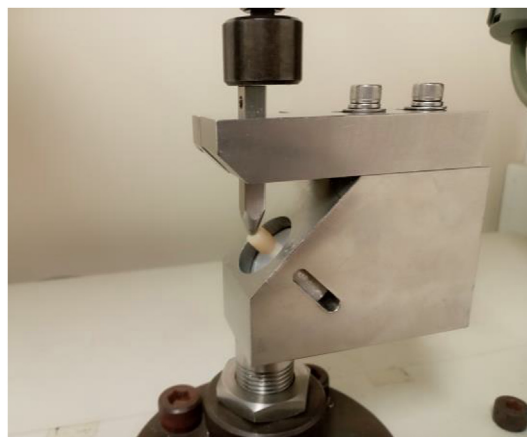
Figure 4 Experimental set up for the fracture test.
