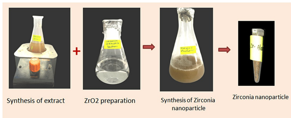
FIGURE 1: Green synthesis of zirconia nanoparticles
