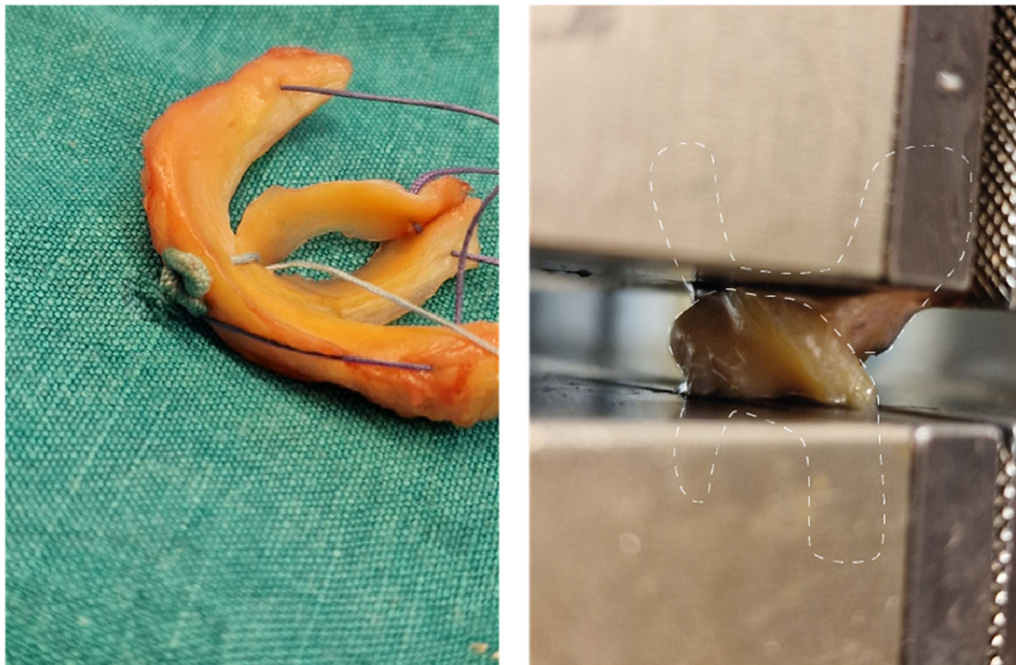
FIGURE 2 Meniscus preparation with all-suture anchor (left). Setup for biomechanical testing, dashed lines depict the outlines of the inner and outer part of the meniscus (right).
