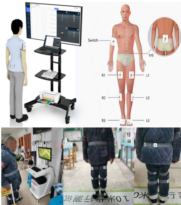
Figure 2 Gait watch, Zhang He Zhi Neng, Guangzhou, China (Gait watch and the position diagram of wearing sensor. Switch: Upper right arm; M0: Upper sacral margin; R/L1: The anterior side of the midsection of the femur; R/L2: Lower edge of the fibula head; R/L3: Behind the metatarsophalangeal joint, the second through the fourth metatarsal bones.
