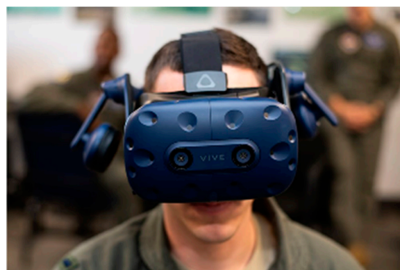
Figure 9. An HTC Vive Pro Eye HR HMD combined with a VOG NET sensor. Taken with permission from [25].
