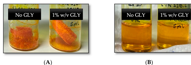
Figure 3. (A) CUR-loaded polymeric micelles visual aspect after lyophilization with 1% GLY and with no GLY; (B) Lyophilized CUR-loaded polymeric micelles with 1% GLY and with no GLY, visual aspect after re-constitution with water/EtOH mixture, followed by co-solvent evaporation.
