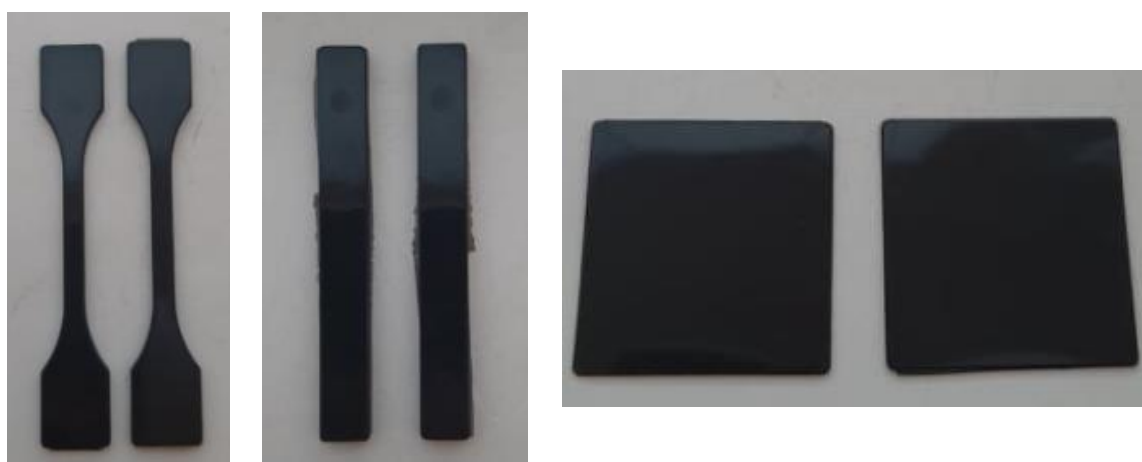
Figure 1. Standard shape 5A (left side) for the elasticity and tensile tests, standard shape 6A (center) for the impact tests, plates from which the discs were cut for the microbiological tests (right side).
