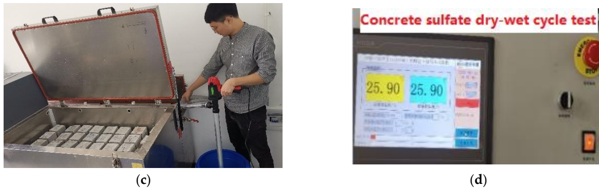
Figure 2. Test procedures. (a) Oven-dry process. (b) Preparation of the test chamber. (c) Liquid drainage from the storage tank. (d) Wet–dry cycling immersion test.
