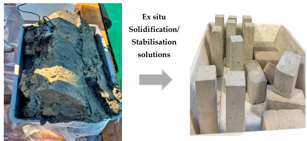
Figure 4. From dredged sediments to prototypes of pavement blocks.
