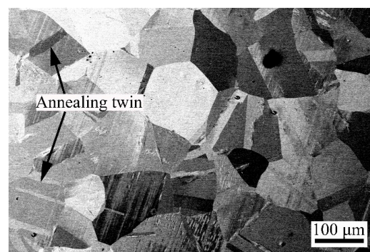
Figure 1. BSEI image of the as-received materials.
