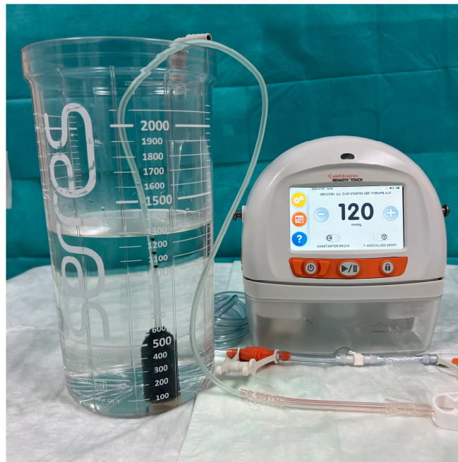
Figure 4. Experimental set-up for comparative measurement of throughput of the two endoluminal vacuum therapy systems (picture created by ME).
