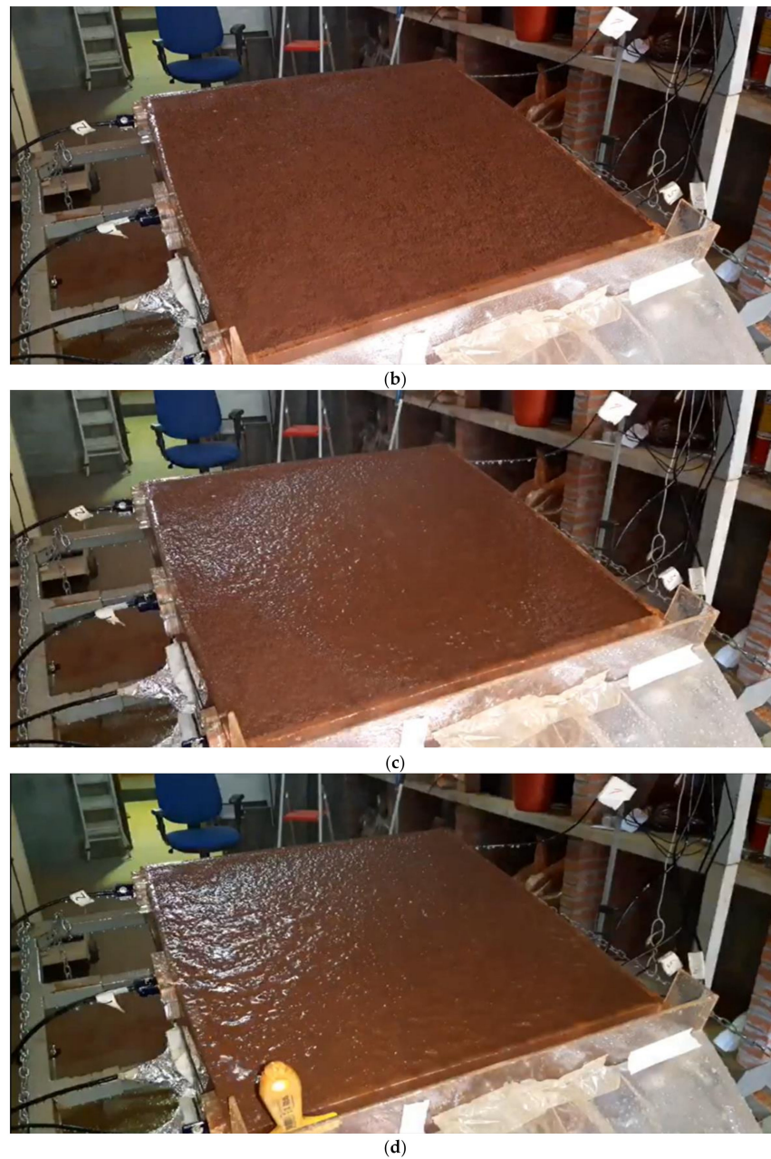
Figure 14. Steps and details of monitoring the test carried out in RS for exposed soil (sample surface). Test considering simulated rainfall of 223.0 \text{ mm h}^{-1} , initial soil moisture of 25%, and \alpha = 15^\circ : (a) overview of the RS before the test; (b) 38 s; (c) 76 s; (d) 152 s after the start of the test.
