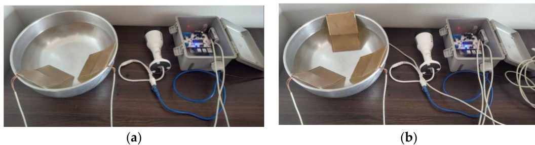
Figure 8. Execution and validation of tests to determine the configuration impedance of rain sensors for different wetting and drying scenarios: (a) two rain sensors; (b) three rain sensors.
