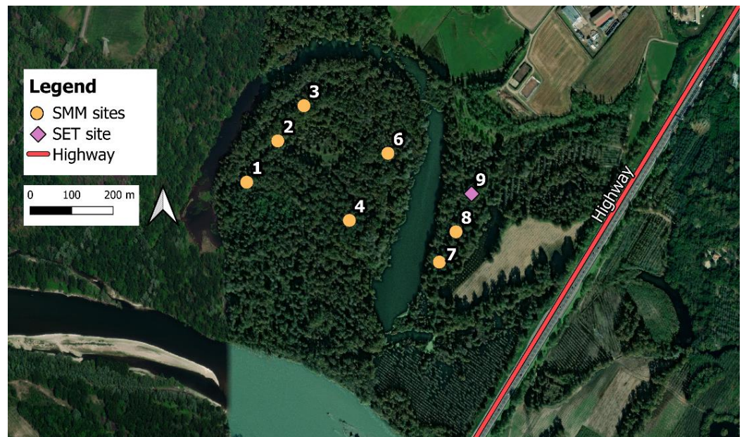
Figure 12. Monitoring scheme at the Ticino Regional Park (Beregardo, PV, Italy). The SMMs are indicated as yellow circles while the SET as a violet triangle. Number 5 is missing due to malfunctioning. The main anthropic noise source (highway) is highlighted in red.
