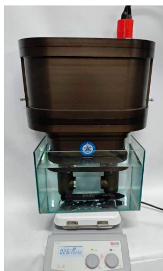
Figure 8. Experimental stability setup for the seawater refractive index measurement system.
