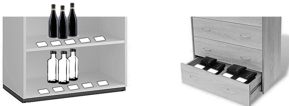
Figure 1. Schematic representation of sections of two of the storage units showing the position of the tag series.
