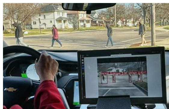
Figure 16. Real-time inference results during the daytime. The proposed system can be run during the daytime and correctly detects pedestrians.
