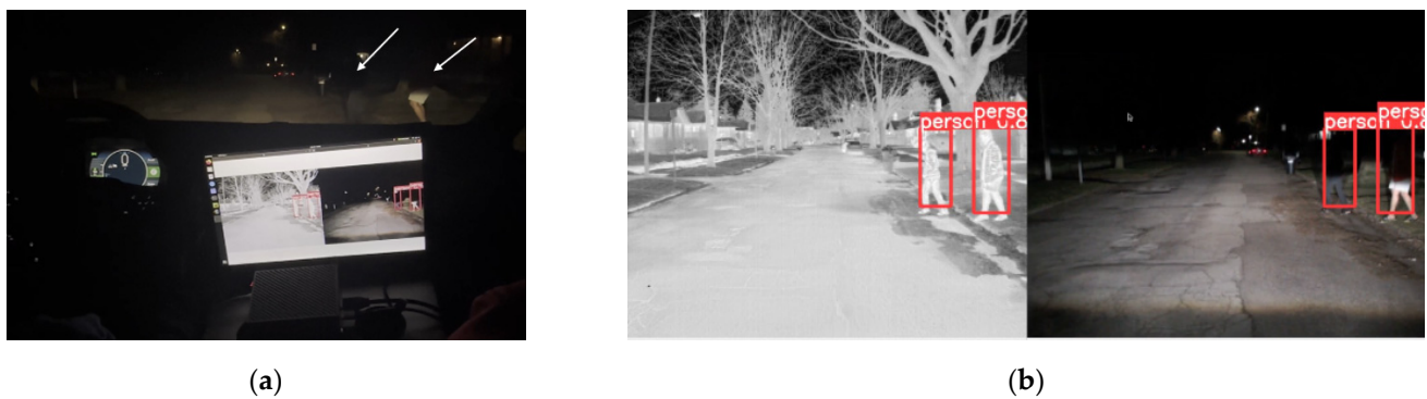
Figure 15. Nighttime testing example 2: (a) Due to the low lighting conditions, two pedestrians on the right side (indicated by white arrows) are not visible. (b) Pedestrians are correctly detected by the sensor-fused system and marked with red bounding boxes on the screen.
