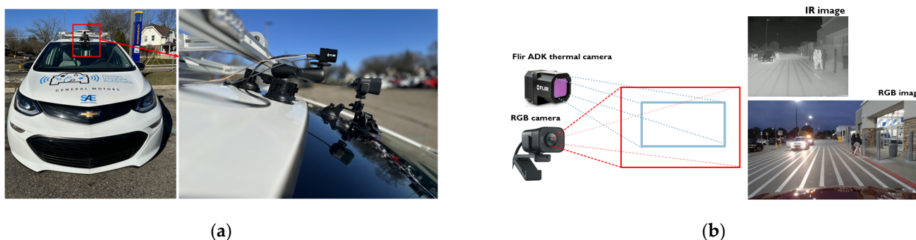
Figure 3. (a) Hardware setup on the testing vehicle; (b) captured images with different FOVs and resolutions.
