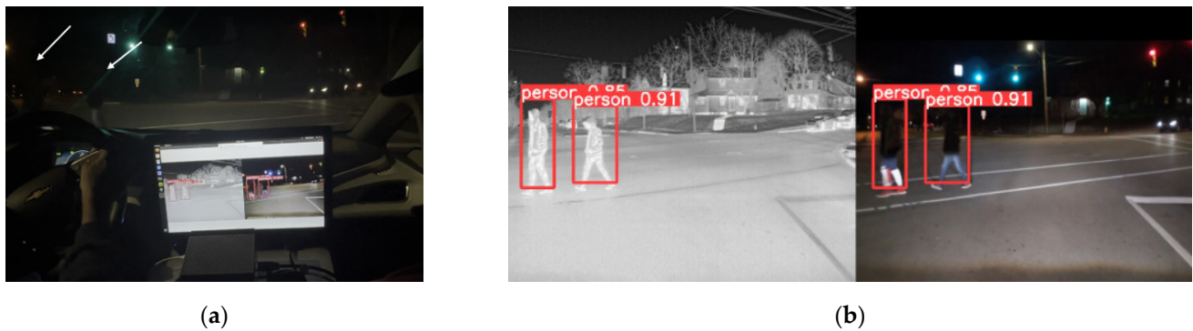
Figure 14. Nighttime testing example 1: (a) Due to the low lighting conditions, two pedestrians on the left side (indicated by white arrows) are not visible. (b) Pedestrians are correctly detected by the sensor-fused system and marked with red bounding boxes on the screen.
