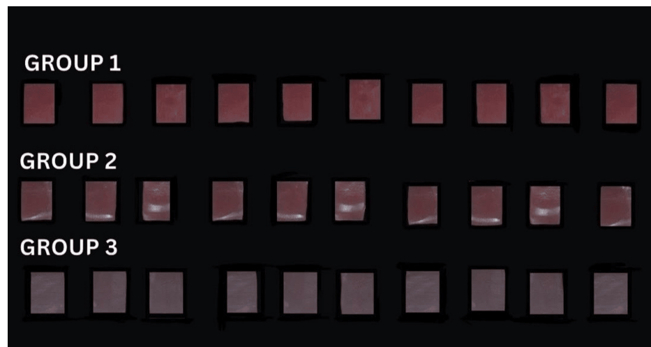
FIGURE 3: Polished specimens. Group 1: milled resin; Group 2: conventional resins; Group 3: printed resin
