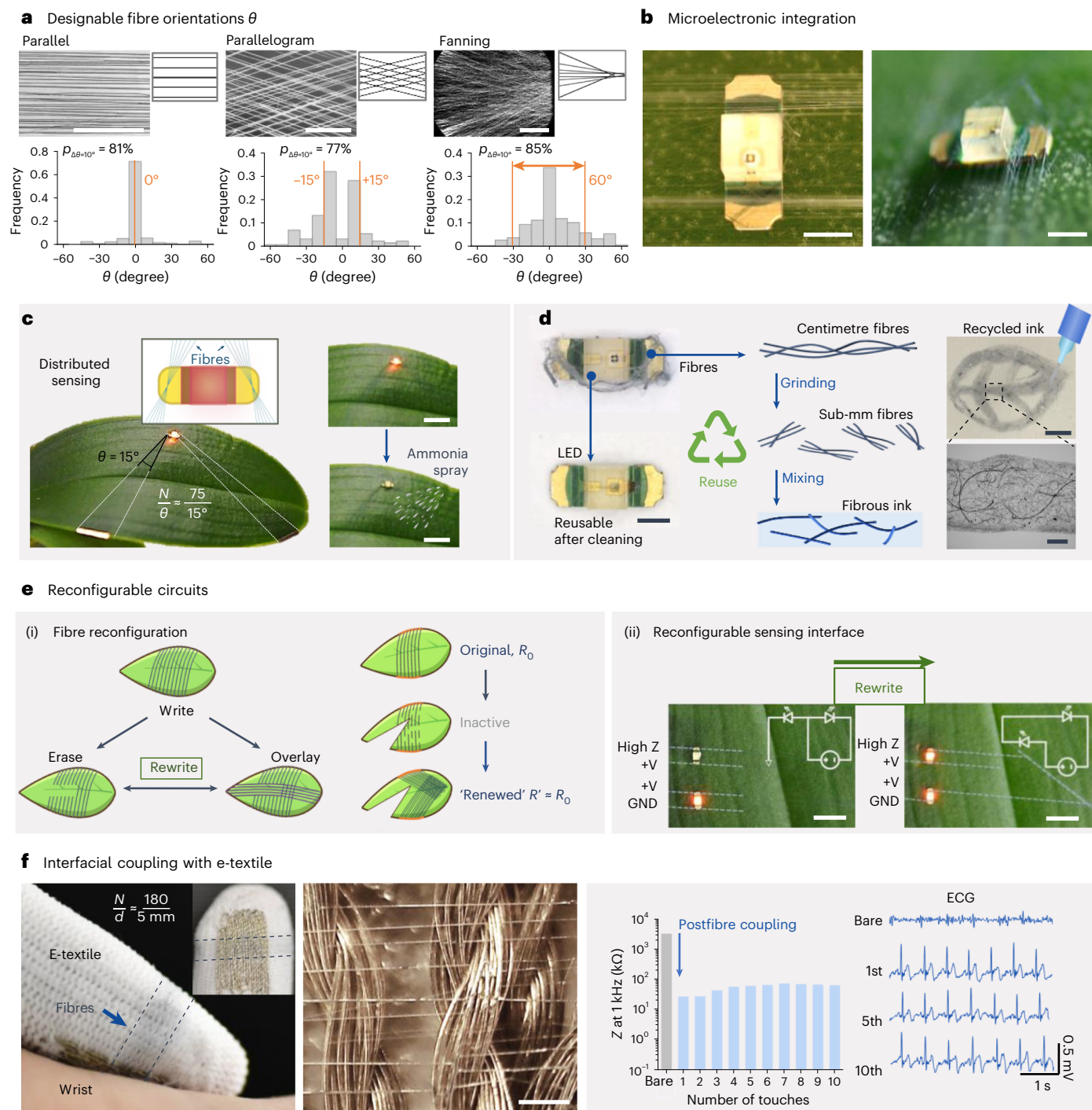
Fig. 5 | Adaptable, versatile and reconfigurable fibre coupling. a , Fibre tethering with designable fibre orientations ( \theta ) is demonstrated by statistical analysis of fibre orientations \theta with different fibre patterns, and the patterning accuracy ( p_{\Delta\theta=10^\circ} ) is calculated by taking an 10^\circ -offset (the width of the binning in the histogram) being an acceptable criterion for misalignment (a horizontal line is used as the 0^\circ baseline for measuring all the fibre orientation angles). b , Photographs showing the top and profile views of fibre arrays connecting to the contacts of an LED (scale bars, 2 mm). c , Distributed bioelectronic fibres to connect with an LED on a plant leaf to warn environmental exposure of ammonia on the plant surfaces (where the dashed lines indicate the boundary of the fibre arrays, scale bars, 5 mm; typical results from independent experiments performed with n > 3 plants). d , Concepts for reusable and recyclable components, where the LED and bioelectronic fibres could be separated: the LED reused, and the fibres recycled into a feedstock to create conductive inks for 3D
