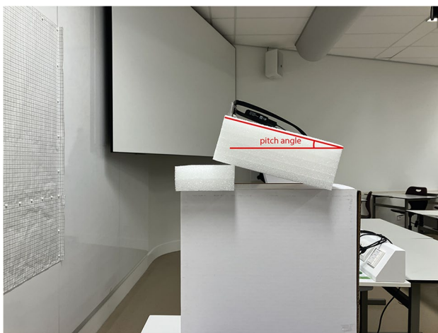
Fig. 7 Setup for estimating the VD parameter. Graph paper consisting of 1×1 cm squares was stuck to the wall, and the Tobii was located at a distance of approximately 1 m from the wall
