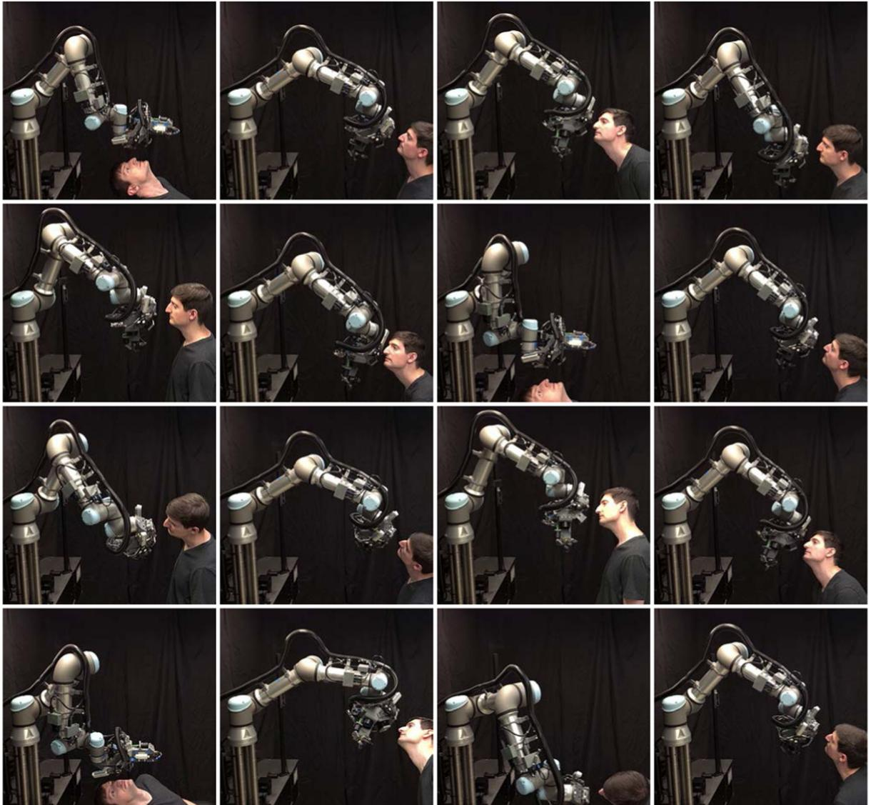
**Fig. 4.** Robotic alignment of OCT scanner with diverse postures (standing, seated, supine) and head orientations (roll, pitch, yaw). OCT imaging is possible for any reachable and collision-free alignment pose.
