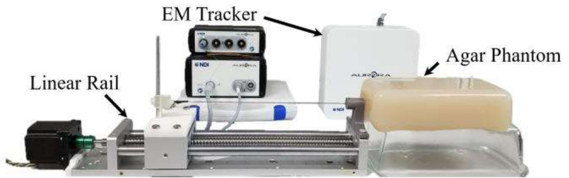
Fig. 5. Experimental setup for empirical validation of the simulation results.
