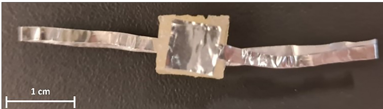
Figure 3. Sample of the fabricated sensing element with terminals. Author photograph
