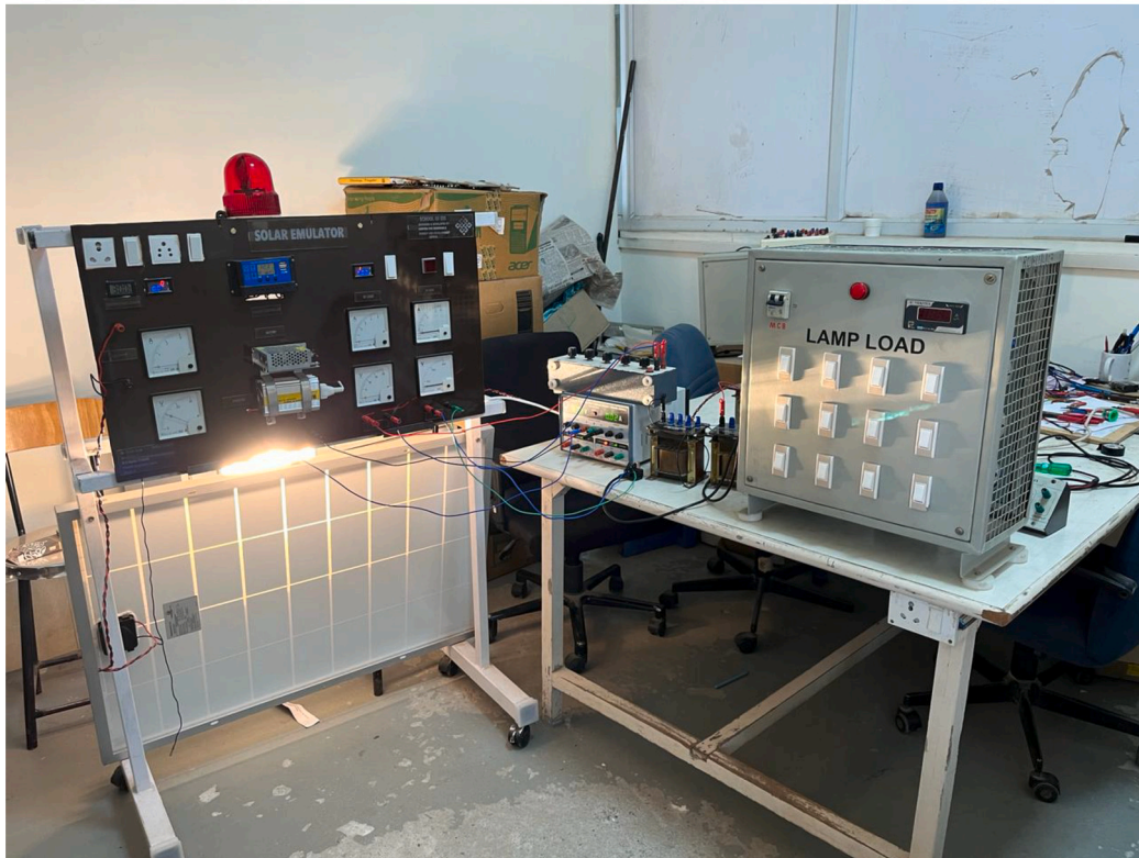
Fig. 3. Microgrid Set Up including Solar PV, Wind and Fuel Cell.
