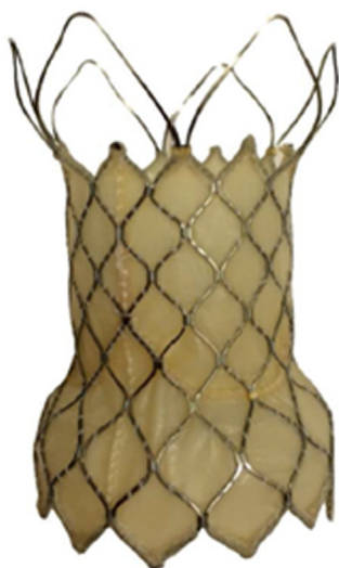
Figure 12. Venus P-valve. Self-expanding nitinol stent with a trileaflet porcine pericardial valve.
